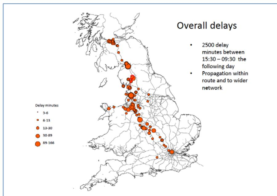
**Figure 1: Propagation of delays from a landslide at Shap, 28th June 2012**
